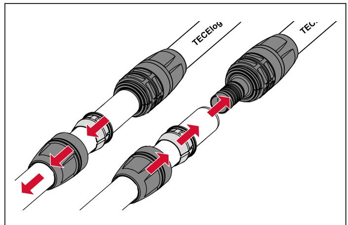
Now push back the collet and clamping ring and pull the pipe away from the fitting base body, then remove the clamping ring and collet from the pipe.
