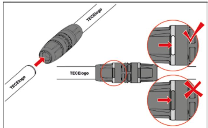
Check the fitting for dirt and clean or swap if necessary. To avoid dirt, do not remove the hygiene caps of the fitting until immediately before the push-fitting operation. Simply push the TECElogo pipe into the fitting until it reaches the stop.
