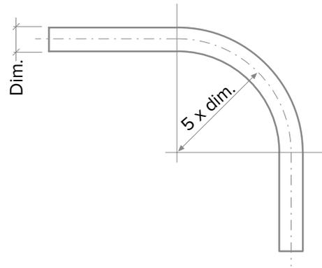
\* without bending spring;  $4 \times \text{dim.}$  with bending spring.
