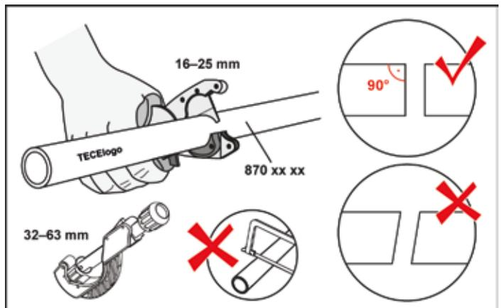
For cutting a TECElogo pipe to length use TECE pipe cutters (order no. 8760002) for the smaller dimensions (up to 25), and use the TECE pipe cutter (order no. 8760008) for the larger dimensions (up to 63)
