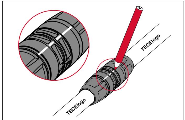
Before undoing a connection, make a continuous marking on the collet and threaded clip. Fix the fitting with the disassembly open-end wrench and unscrew the collet with the dismantling key.
