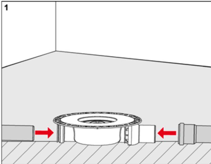
Position drain and connect to wastewater pipe. In the case of drains with a vertical socket, a core hole with a diameter of 130 mm is required.
