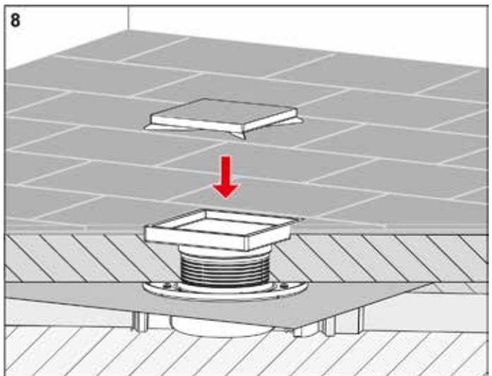
After drying, insert the tileable channel into the grate frame.
