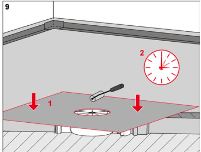
Insert sealing sleeve in fresh coating and press to remove creases. Allow coating to dry.
