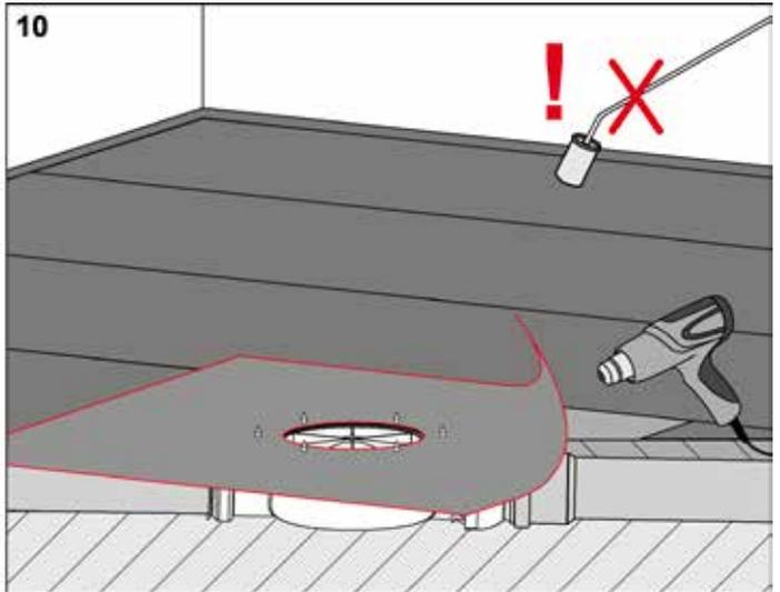
Weld the cut-to-size sealing foil with the sealing strip.
