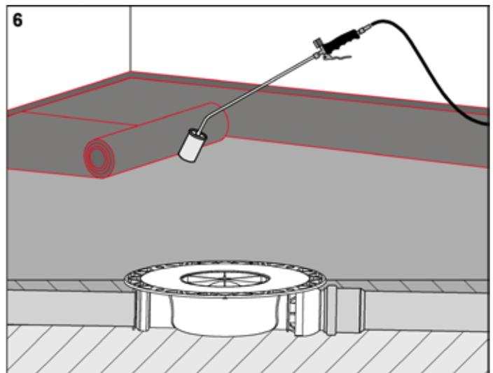
Apply sealing strips (bitumen/EPDM) in accordance with the manufacturer's instructions.
