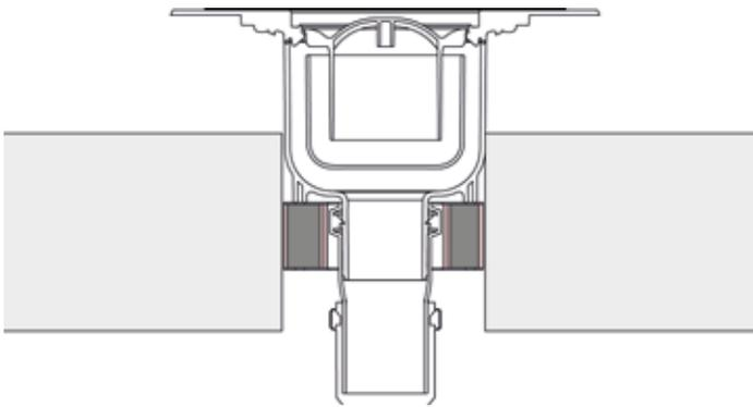
As temperatures rise during a fire, this material foams up to many times its original form. This causes the remaining annular gap towards the core hole on the outside of the fire protection sleeve to close.
