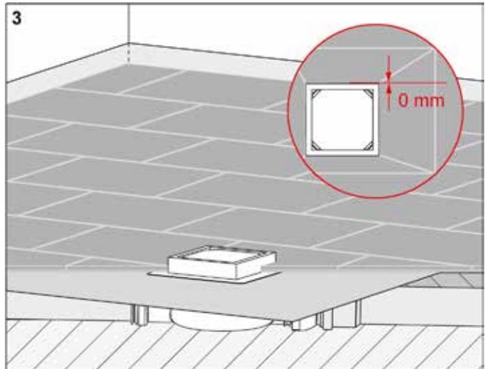
Mount the floor covering without any distance between the bare-wall protection.
