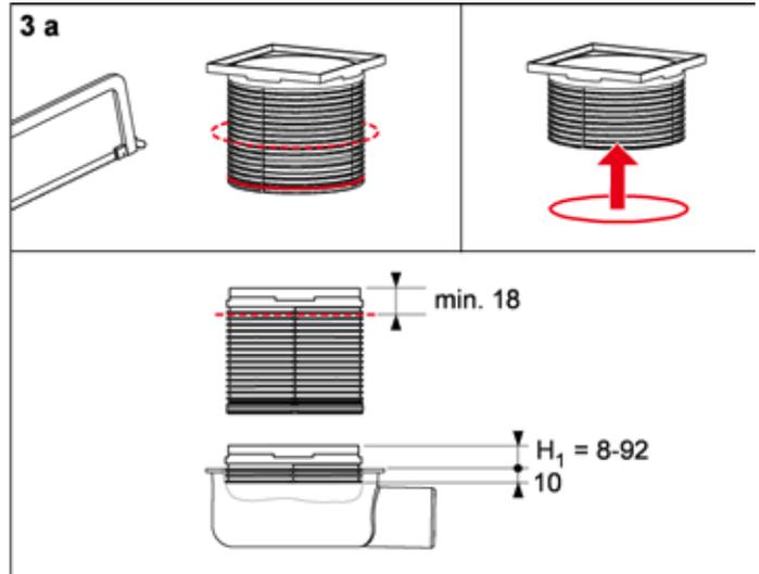
The drain top must be cut to length, the O-ring seal should sit in the lowest groove.
