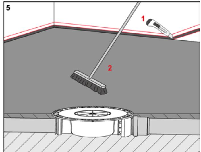
Once dry, cut off the excess edge insulation strips and PE foil, clean screed.
