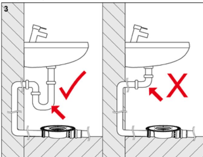
If a lateral inflow is used, an odour trap is required in the inlet pipe.
