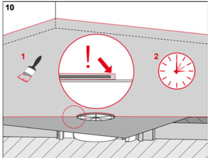
Apply second sealing coating over complete area: The sealing sleeve must be completely covered by the damp-proof coating. Allow coating to dry.
