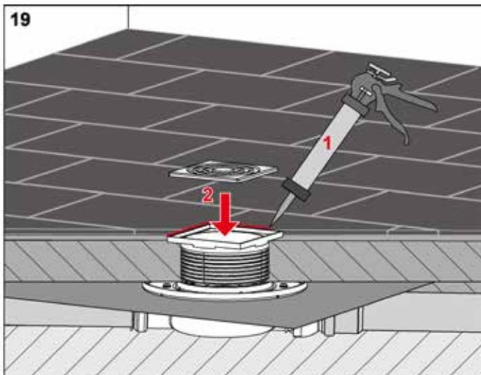
Seal the joint with permanently elastic material and install the grate.
