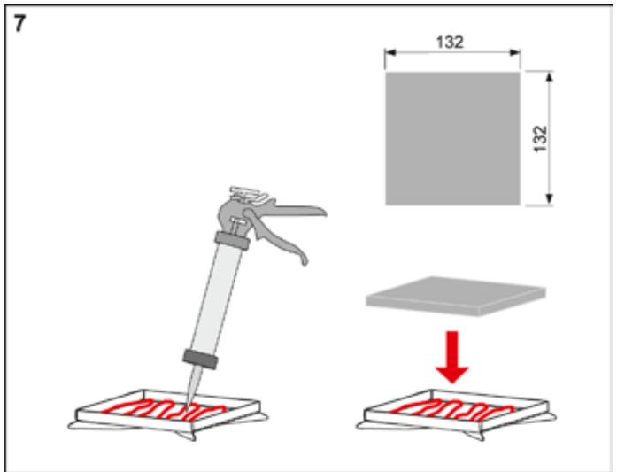
Cut the floor covering (approx. 132 x 132 mm) and bond in the tileable channel with flexible adhesive (e.g. silicone or epoxy resin adhesive).
