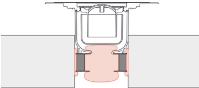
In the socket area, the outflow nozzle including the pushed-on HT pipe sleeve becomes crushed.
