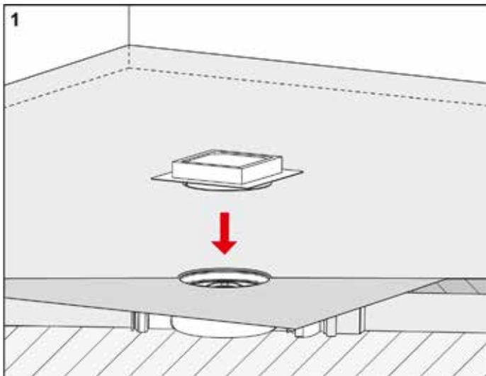
Insert the grate frame with the bare-wall protection into the drain, and align.
