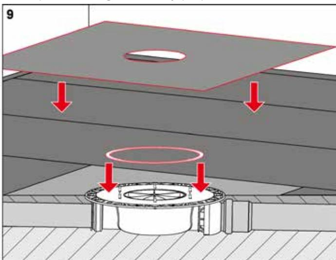
Apply seal and accurately cut the sealing foil (EPDM) to size.
