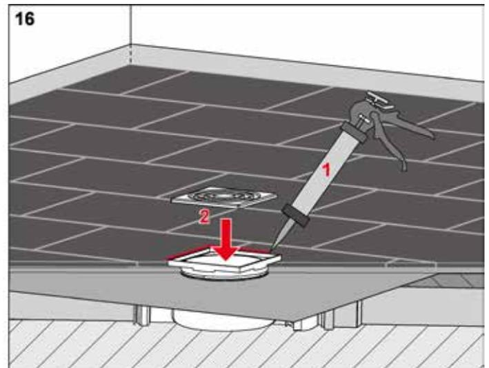
Seal the joint with permanently elastic material and install the grate.
