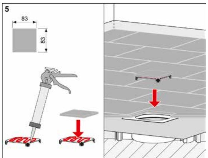
Cut the floor covering (approx. 83 x 83 mm) and bond to the support with flexible adhesive (e.g. silicone or epoxy resin adhesive). After drying, insert the tile base into the grate frame.
