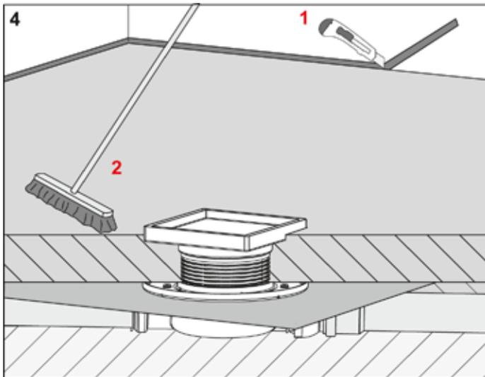
Once dry, cut off the excess edge insulation strips and PE foil, clean screed.
