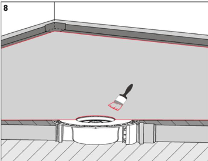
Apply first sealing coating over complete area.
