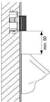
When positioning the cistern, observe the distance to the urinal ceramic. For aesthetic reasons, we recommend that the distance to the cistern is no less than 50 mm.
