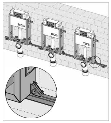
TECEbox series installation – with TECEprofil tube and corner joints
