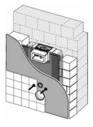
The thickness of the wall must be at least 18 mm but no more than 100 mm. See the section on flush plates for information about the wall structure required for the respective flush plate.
