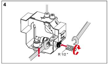
To connect the pipe, hold the connection housing as shown in fig. 4.
