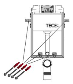
The module must be completely bricked into the wall and all remaining hollow spaces must be filled in. Install the bare-wall protection and the threaded rods.
