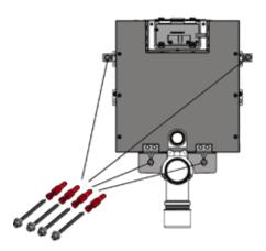
Set the required distance to the wall at the four depth-adjustable positions.
