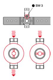
Fit the bare-wall protection and make sure that it is aligned correctly.
