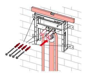
The distance from the threaded rods to the washstand ceramic retainer can range between 170 and 280 mm.
