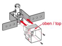
The bare-wall protection housing is cut off flush to the wall after tiling.
