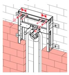
After installation and connection of all connection pipes, the module is bricked in.
