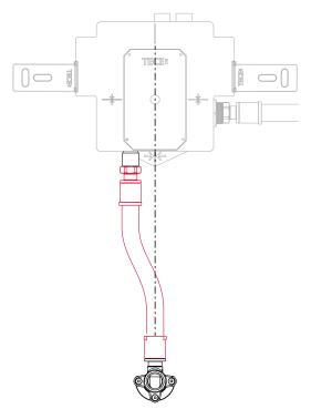
Any approved pipe systems can be used for the water connection and inflow for the urinal ceramic. Make sure that the inflow for the urinal ceramic is positioned centrally beneath the urinal flush valve housing.
