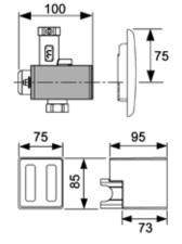
The flush valve housing is placed in a wall recess and attached using the retaining plate. Any approved pipe systems can be used for the water connection and inflow for the urinal ceramic.
