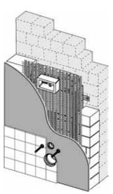
The thickness of the wall must be at least 18 mm but no more than 100 mm. See the section on flush plates for information about the wall structure required for the respective flush plate.
